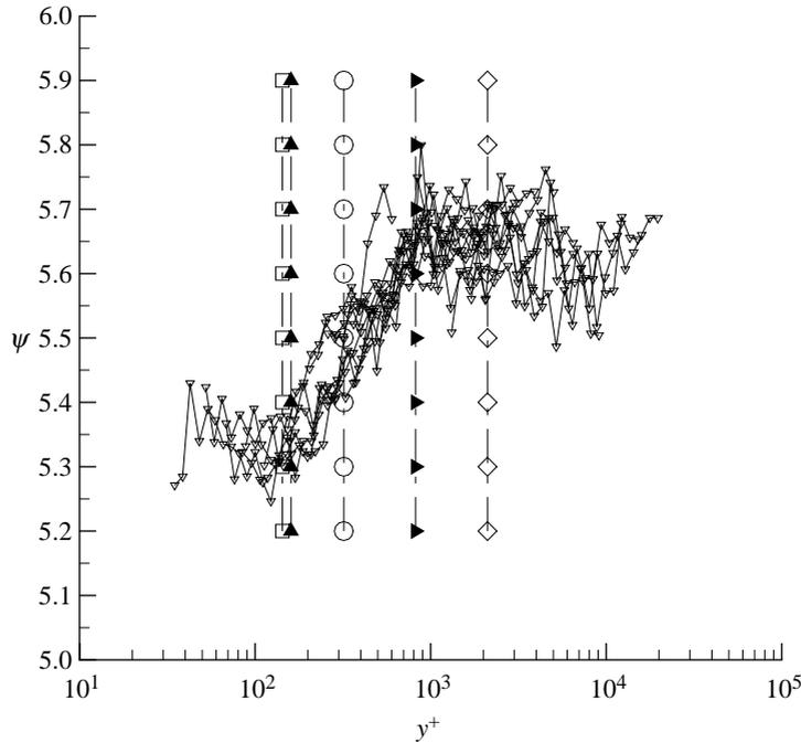
Figure 3. Mean velocity deviation,  $\psi$ , from the log law with  $y^+$  for  $y/R < 0.12$ .
