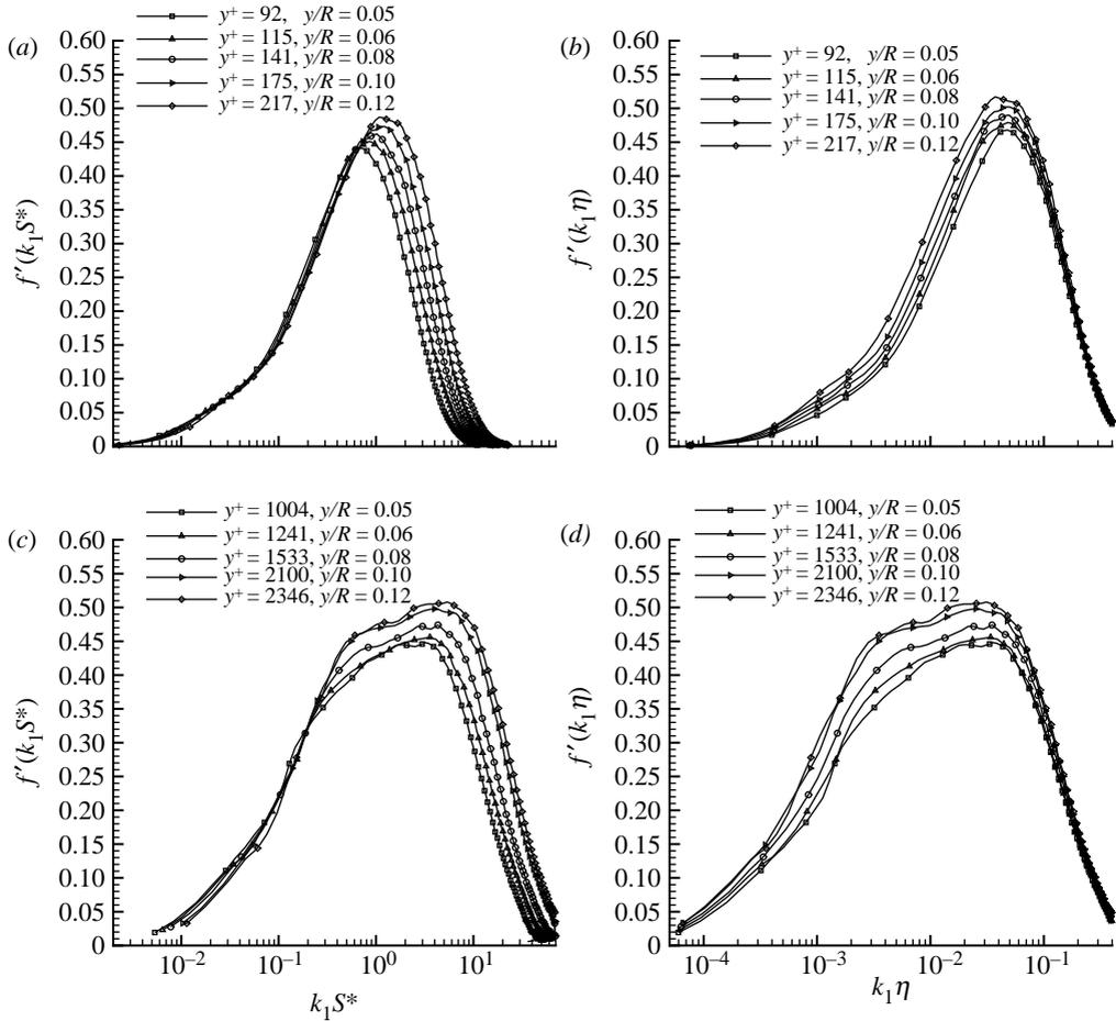
Figure 6. Pre-multiplied spectra in the overlap region using shear and Kolmogorov scaling, (a, b)  $Re_D = 75 \times 10^3$  and (c, d)  $Re_D = 1.0 \times 10^6$ .
