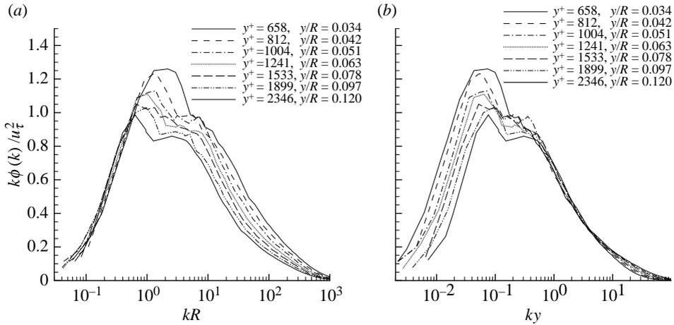
Figure 4. Compensated spectra at  $Re_D = 1 \times 10^6$  in (a) outer and (b) inner scaling.
