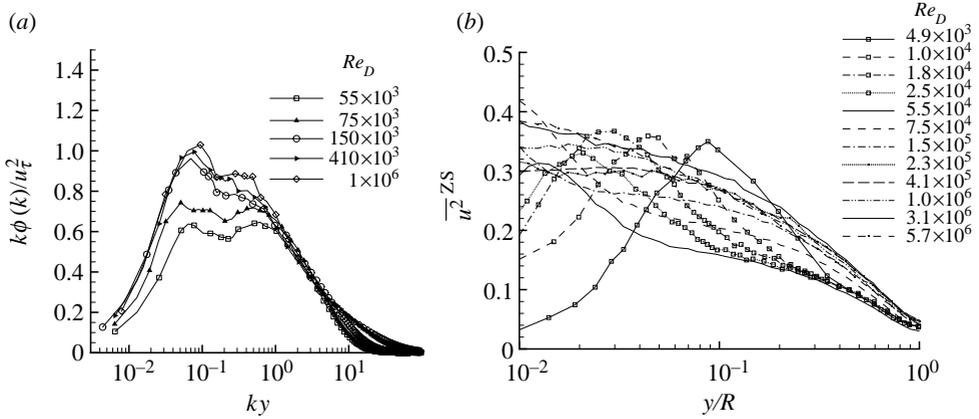
Figure 5. (a) Compensated spectra in inner scaling at constant wall-normal position  $y/R=1$ , various Reynolds numbers and (b) variation of  $\overline{u^2}$  in ZS outer scaling (low Reynolds number data  $4.9 \times 10^3 \leq Re_D \leq 25 \times 10^3$  from den Toonder & Nieuwstadt (1997)).
