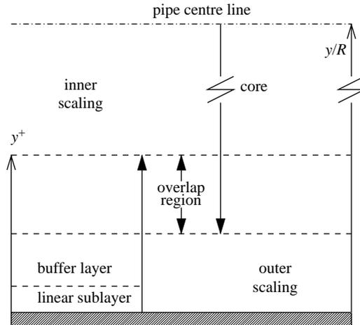
Figure 1. Schematic of mean velocity scaling in fully developed pipe flow.
